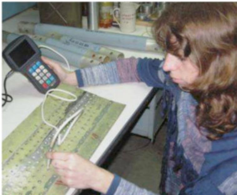
Fig. 1. Practicing of local corrosion damages detection technique
